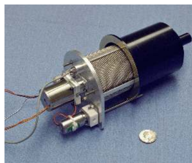
Absorption compressor designed for Mars ISRU. Photo: NASA / ARC
