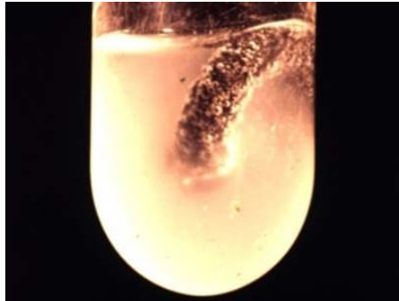
Elastomer o-ring dissolving in supercritical CO 2 Photo: Martyn Poliakoff
